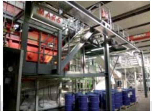
The MARS® plant: the new conveying technology can be seen (white), the water-cooled pipes for the grate (green), and the combustion chamber (red)
