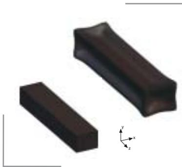
Calculation of the dimensional changes of a rectangular seal profile (L x W x H = 300 x 25 x 20 mm), which is typically used for the sealing of wall/floor joints in the construction industry (concrete construction), after 17 days of swelling.
