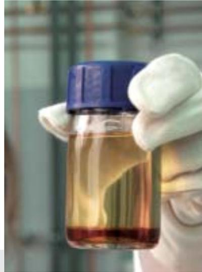
Nitrogen-containing catalysts accelerate the phase separation and product processing for biodiesel synthesis
