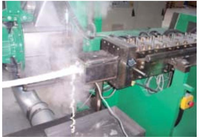
Extrusion plant for corn starch
