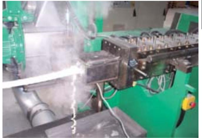
Extrusion plant for corn starch
