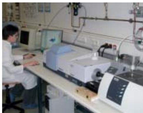
Coupled thermogravimetry/infrared spectroscopy (TG-IR)
